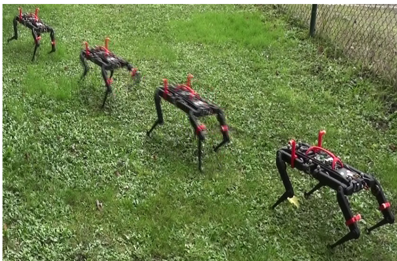
Figure 11.2: Trotting gait on wet grass. Connection with the robot was done by Wifi with the same computer than we used indoors. Previous experiments showed that packet loss did not hamper the behavior for distance under 25 m.
