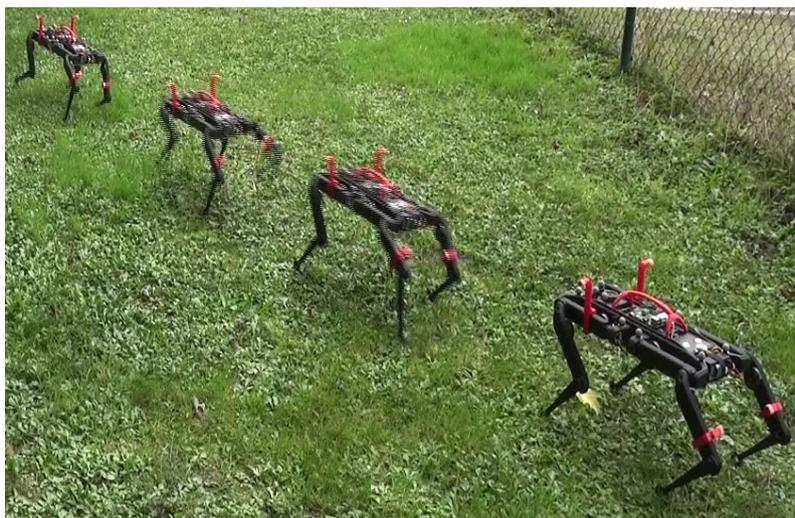
Figure 11.2: Trotting gait on wet grass. Connection with the robot was done by Wifi with the same computer than we used indoors. Previous experiments showed that packet loss did not hamper the behavior for distance under 25 m.
