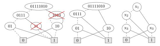
Figure 3.1: The binary decision diagram for Boolean function  $g_1(x_1, x_2, x_3)$ .
