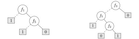
Figure 2.4: Two optimal decision trees in size 5 and 7 maximising examples for the dataset in Table 2.5.
