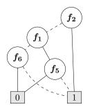
Figure 1.4: The Binary Decision Diagram of max depth 4 classifying all examples.
