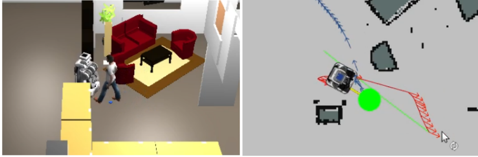
Figure 2.8: Narrow passage passing scenario. In this scenario, the human and robot arrive at the common passage at the same time, and one should back off to provide a way for another. Otherwise, there exists no solution. This is one of the intricate situations addressed in this work, and the picture on the left shows the simulation of this scenario in MORSE. The right side picture shows the trajectories for the human (blue) and the robot (red), generated using the proposed framework, HATEB-2. It can be seen from the picture that the robot’s trajectory (red) is making the robot move backwards and hence providing a way for the human.
