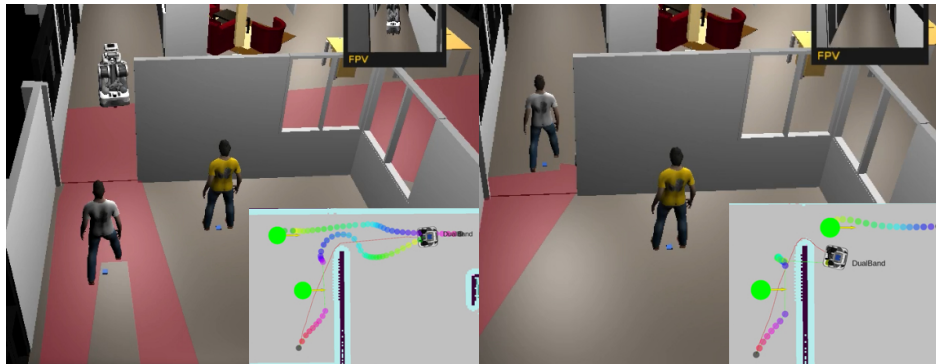
Figure 3.4: Door crossing scenario in the simulated environment. The human moves towards the door. The robot sees the human and waits on the side of the door (right) until the human crosses.
