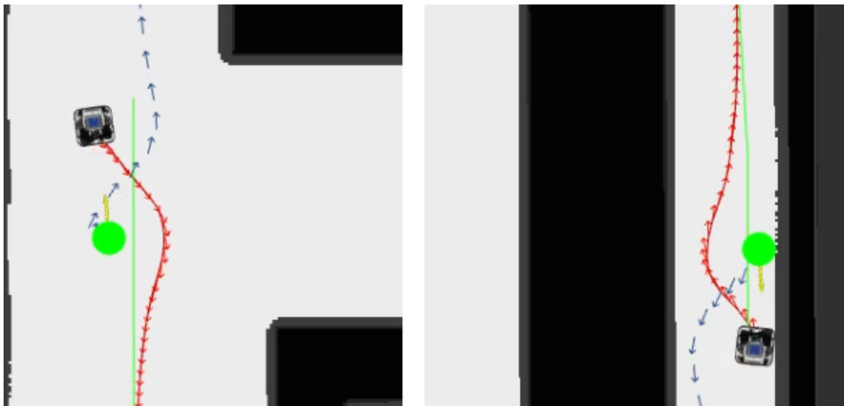
Figure 2.1: Robot getting stuck due to entanglement of trajectories. The poses in blue correspond to the human’s trajectory and the ones in red to the robot’s trajectory. In the situations shown, there exists an alternate solution for the robot to solve the problem. However, the assumption about the human having non-zero velocity and the safety constraint makes the robot wait in the same entanglement, speculating the motion of the human. The picture on the left is of open space, whereas the one on the right is of a narrow corridor.
