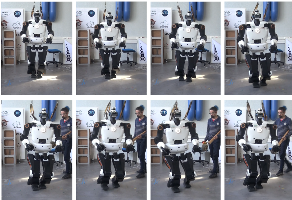
FIGURE 6.8: Snapshot of the push recovery experiment. The robot walks without disturbance in the first 4 images, then gets pushed by a stick and recovers from the fall by stepping aside. The push happens approximately in the lower left frame, at t \approx 17.5 s. The video of the experiment is available at https://peertube.laas.fr/w/gtbFKTS8TA6wtwegeSrrBt
