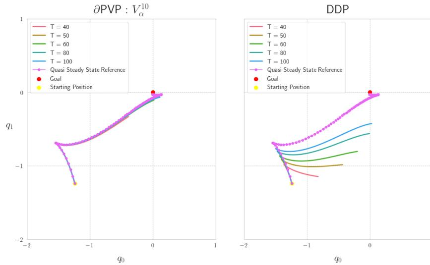
**Fig. 5.7.:** State trajectories computed by  $\partial PVP_v$  and DDP for different initial preview horizons  $T$ .
