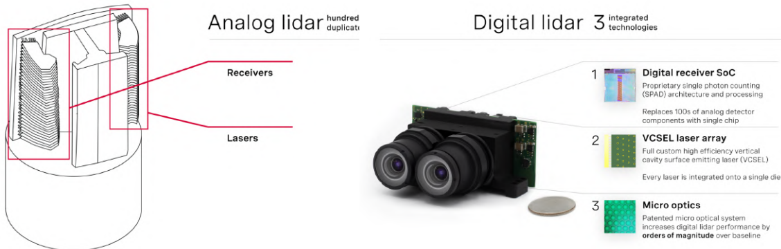
Figure 2.14: Comparison between analog and digital LiDAR architectures, excerpt from [38].
