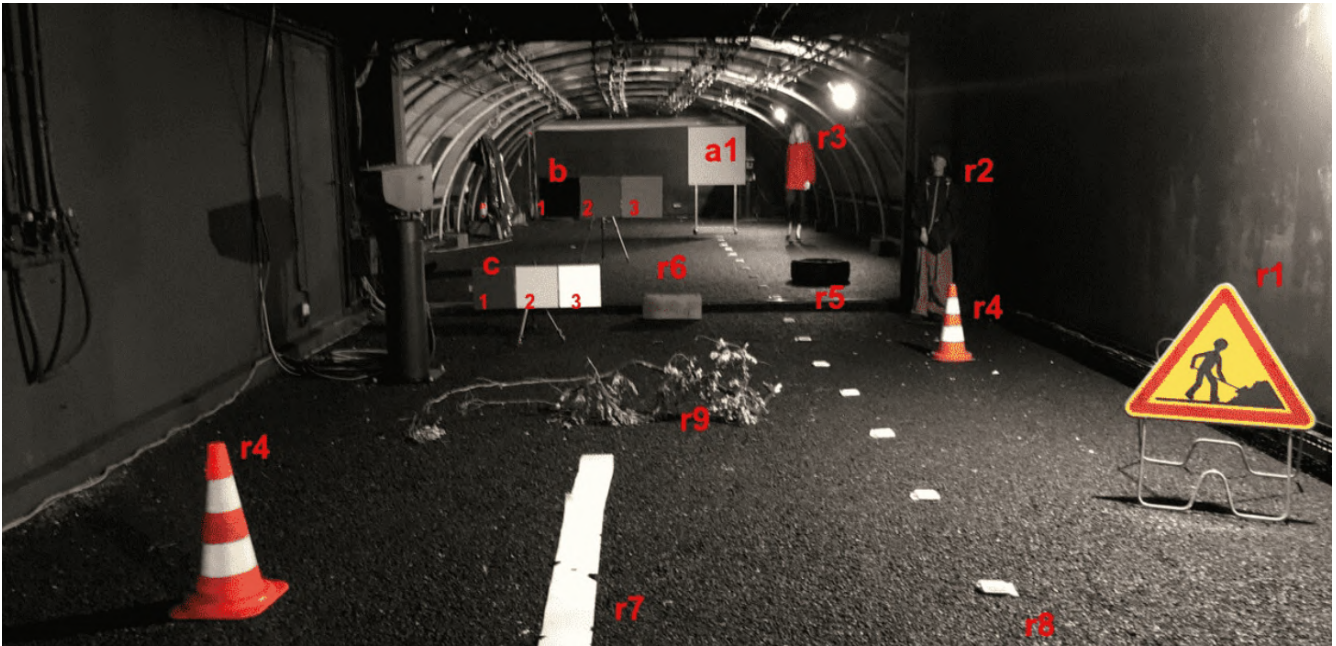
Figure 6.5: Inside of the climatic chamber during the experiments, with targets denoted by labels.
