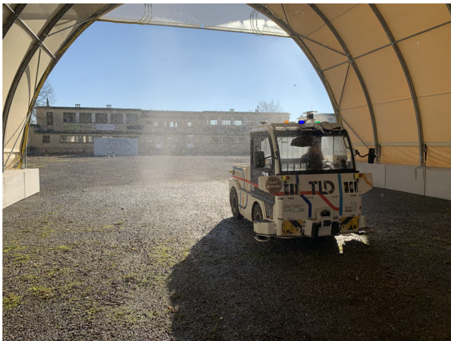
Figure B.1: EasyMile TractEasy under the rain tunnel.
