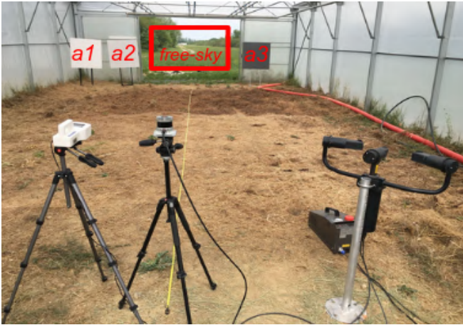
(a) Sensors and targets layout in the artificial fog experimental setup. a1 , a2 , and a3 targets in decreasing reflectivity order. At the entrance, from left to right: the PSD sensor, the OS1-128 LiDAR, a Biral VPF700 scatterometer, and the smoke machine.
