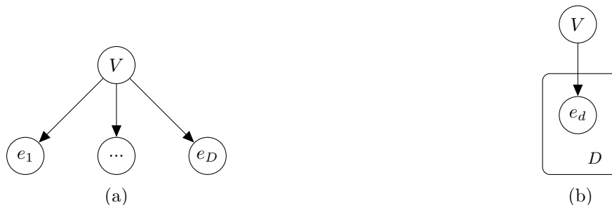
Figure 7.1: Probability Graphical Models (PGMs) of the naive Bayes classifier model for visibility classification using independent LiDAR echoes, related to eq.7.2. (a): developed model, (b): same model using the plate notation.
