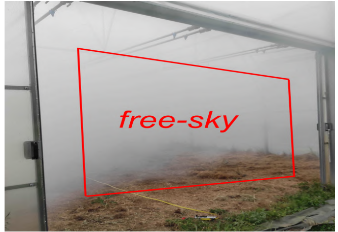
(b) Illustration of the free-sky target during a smoke dissipation with opened rear-doors. Note that the smoke is not uniformly distributed in the chamber during dissipation and evacuates mainly through the top of the chamber.
