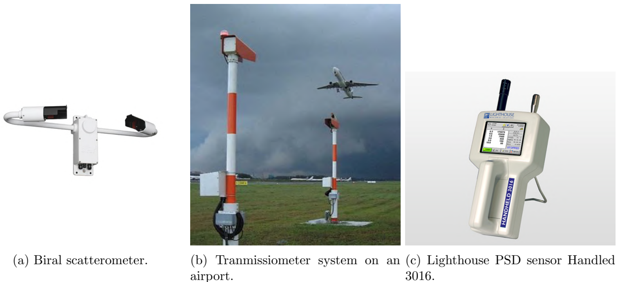
Figure 3.4: Pictures of visibility and PSD sensors.
