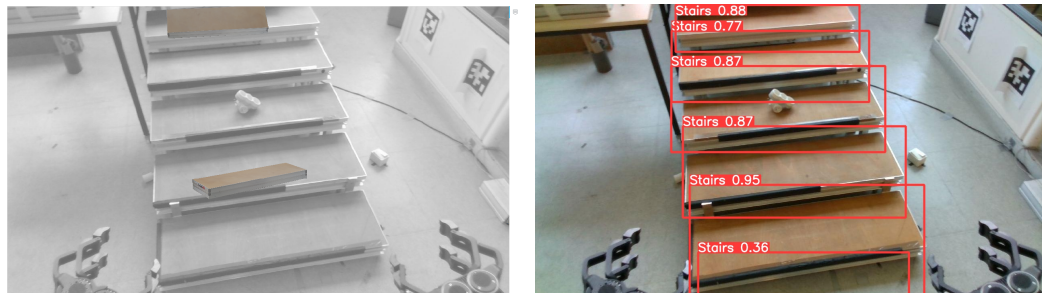
(b) Comparison of the results from CosyPose and YOLO in the case of messy objects.
