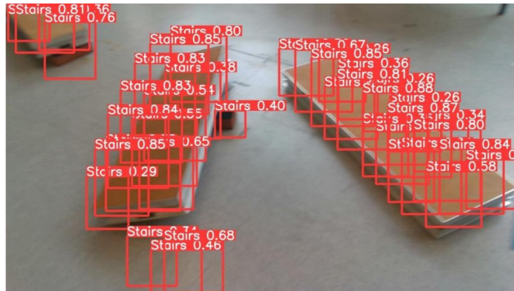
Figure 5.9: Example of the detection of the stairs with the first trained YOLO model.
