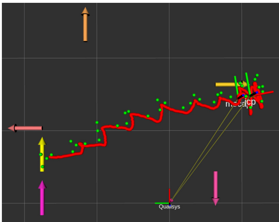
Figure 2.8: Visualization of the recorded data on Rviz (in red the MoCap set and in green the ICP set)
