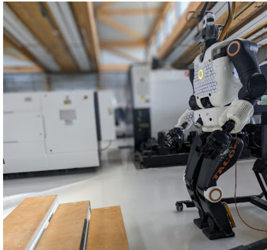
Figure 6.1: The Talos robot with the depth camera added to its waist.
