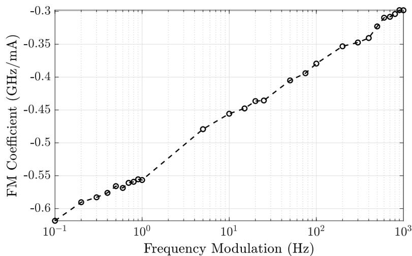
Figure 3.12: Experimental measurement of FM coefficient as a function of modulation frequency.
