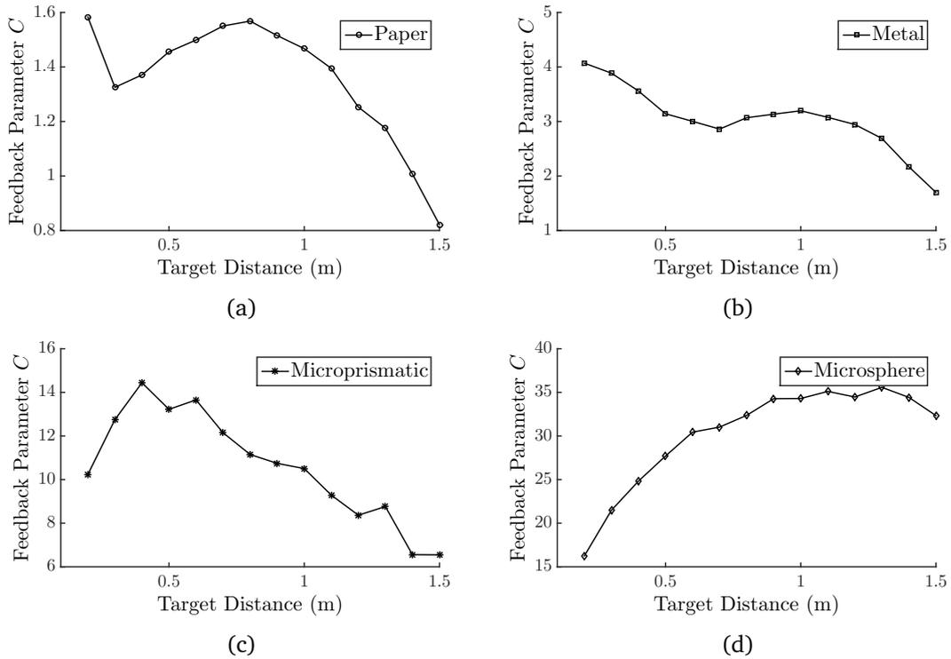
Figure 3.9: Variation of feedback parameter  $C$  as a function of the external cavity  $L_{\text{ext}}$  with different target's surfaces. (a) White paper. (b) Metal. (c) Microprismatic reflective tape. (d) Microsphere reflective tape.
