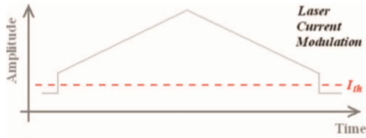
Figure 1.19: The shape of laser current modulation [9].
