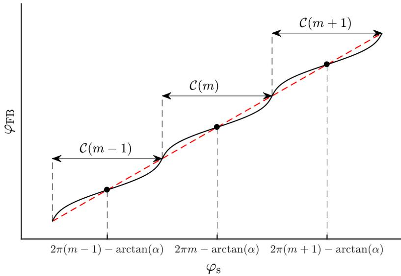
Figure 2.4: Plot of the excess phase equation for  $C = 0.7$ , and  $\alpha = 5$ . The red broken line is the axis where there is no optical feedback, and the black solid line indicates the solution path of  $\varphi_{\text{FB}}$ .
