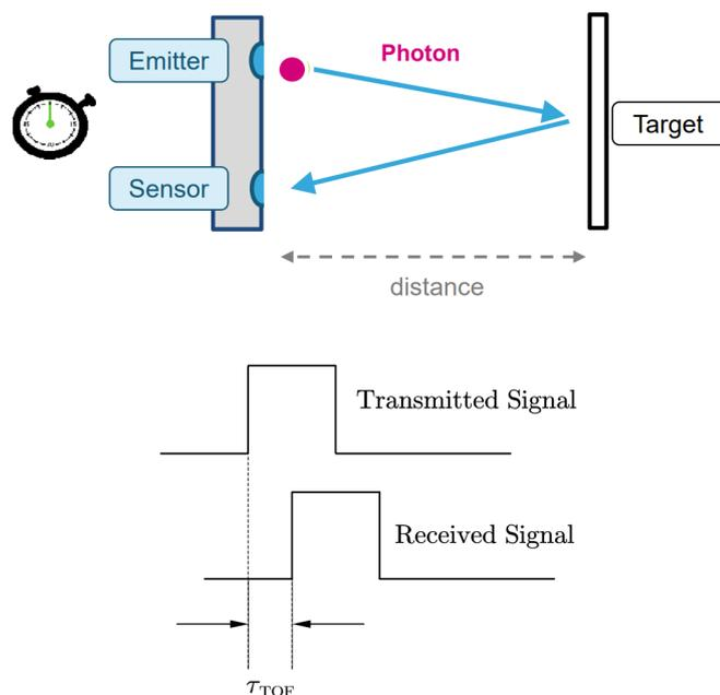
Figure 1.5: Principle of direct TOF distance measurement method [2].
