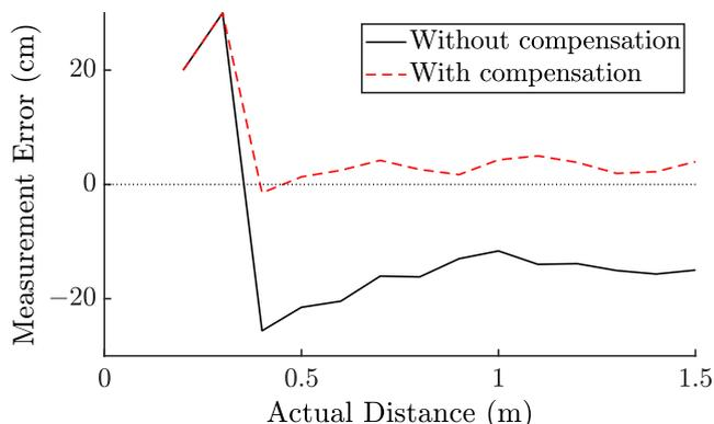
Figure 3.29: Measurement error with time spacing method: the solid black line measured with  $\Omega = -354$  MHz/mA and the solid red line measured with the exponential of the FM coefficient resulting from the fringe frequency under the weak optical feedback regime.
