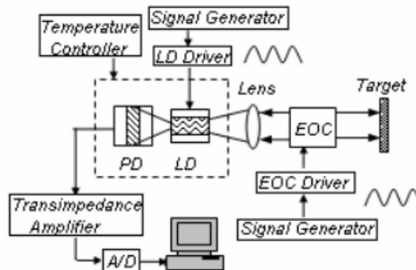
Figure 1.16: Experimental setup with double modulation—wavelength and phase [7].
