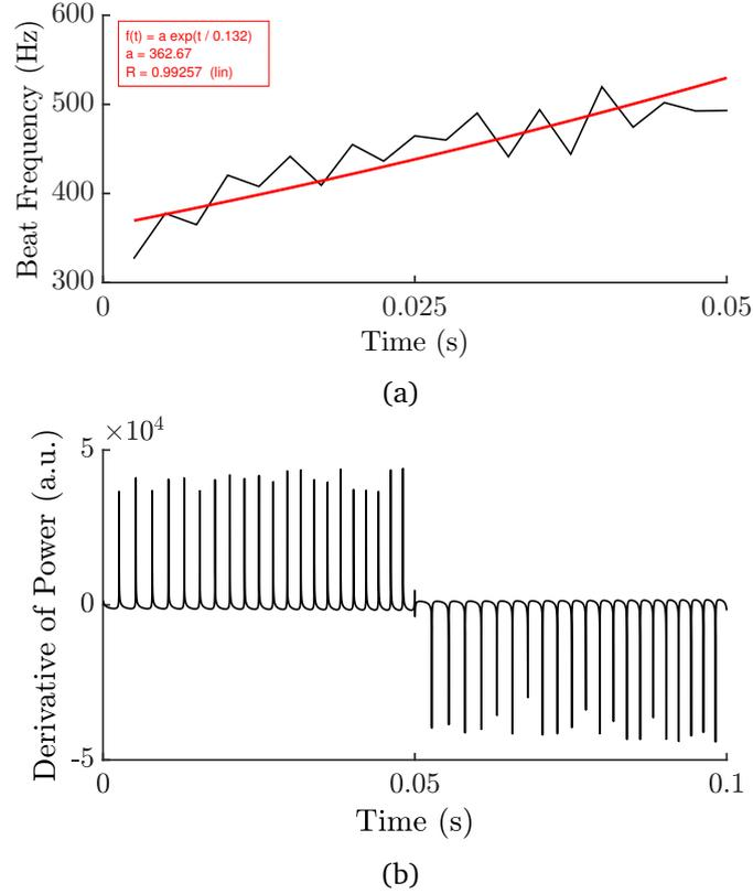
Figure 3.17: (a) Plot the measurement result of fringe frequency indicated in black solid lines and the curve fitting from MATLAB Toolbox indicated in the red solid line. (b) Plot SMI absolute distance with the obtained parameters in (a) under the optical feedback level  $C = 0.9$ .
