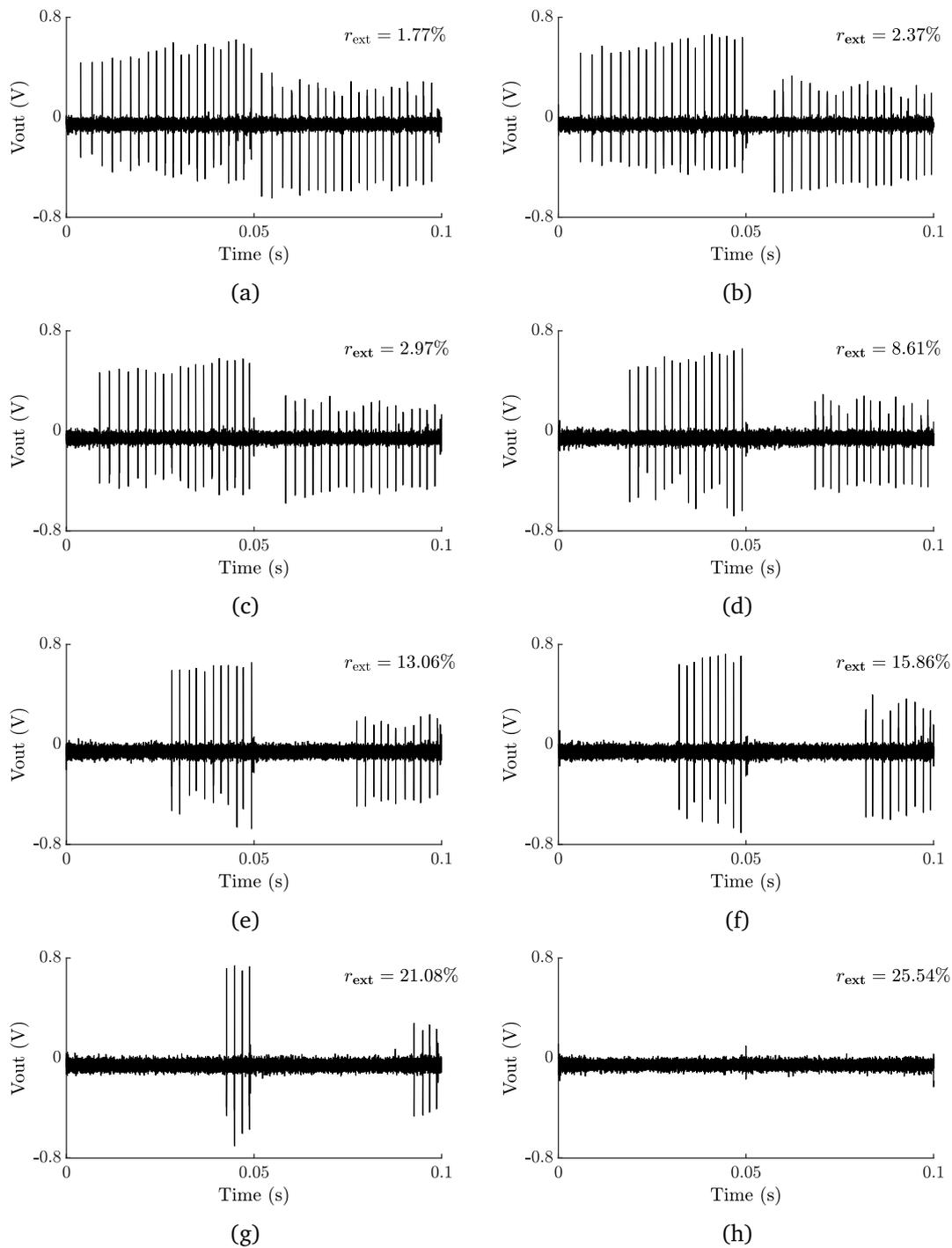
Figure 3.19: Experimental SMI signal acquisition for the distance of 1.5 m with different target's amplitude reflectivities. (a) 1.77%. (b) 2.37%. (c) 2.97%. (d) 8.61%. (e) 13.06%. (f) 15.86%. (g) 21.08%. (h) 25.54%.
