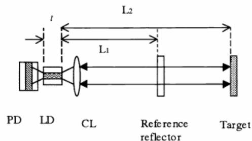
Figure 1.12: Self-mixing interferometers with double external cavities [5].
