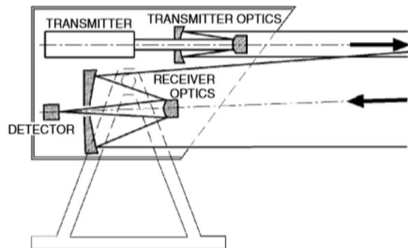
Figure 1.4: Essential optical components of a LiDAR system [1].
