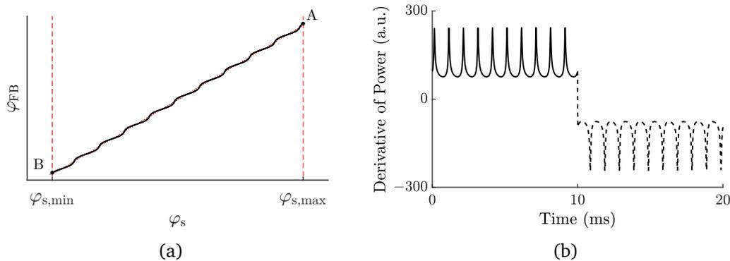
Figure 3.2: The behaviour of the laser diode phase under weak optical feedback  $C = 0.7$ . (a) Plot phase response in function of phase stimulus. (b) Plot the derivative of output power resulting from the dwelling stable solution from (a).
