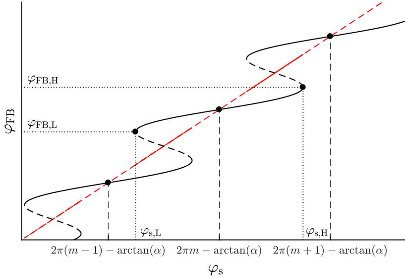
Figure 2.6: Plot of the excess phase equation for  $C = 3$ , and  $\alpha = 5$ . The red broken line is the axis where there is no optical feedback, and the black solid and broken lines indicate the region of stable and unstable solution of  $\varphi_{FB}$  respectively.
