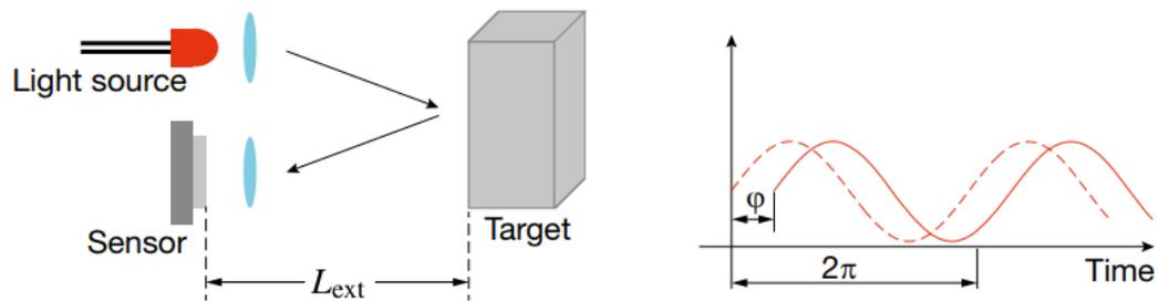
Figure 1.6: Principle of phase-shift distance measurement method [2].
