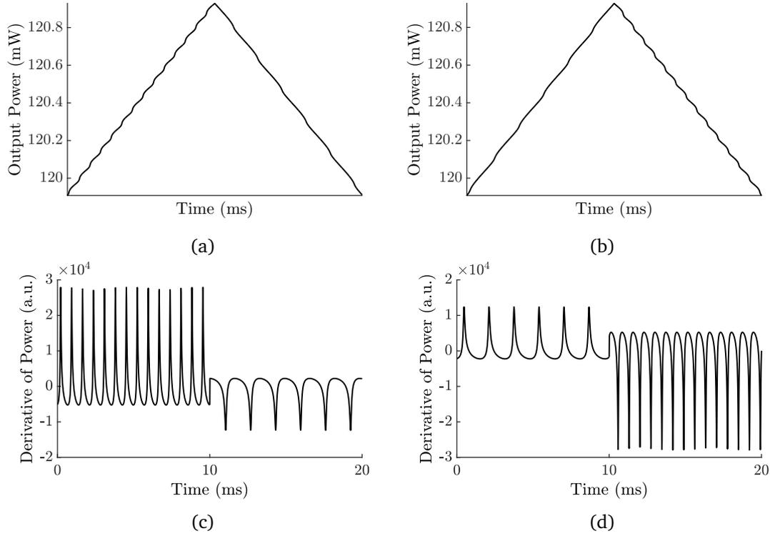
Figure 4.9: Simulation self-mixing power resulting from modulating the phase stimulus in the triangle waveform under the feedback parameter  $C = 0.7$  in different velocity directions. (a) In the clockwise direction with the speed  $v = +0.35$  mm/s. (b) In the anticlockwise direction with the speed  $v = -0.35$  mm/s.
