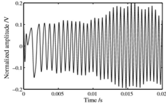
Fig. 4. SMI signal in one tuning period.
