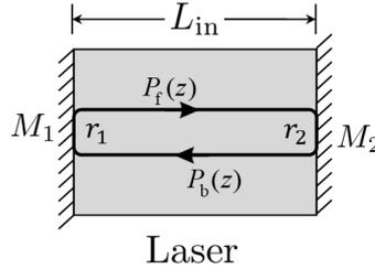
Figure 2.1: Schematic of two-mirror model of an optical cavity.
