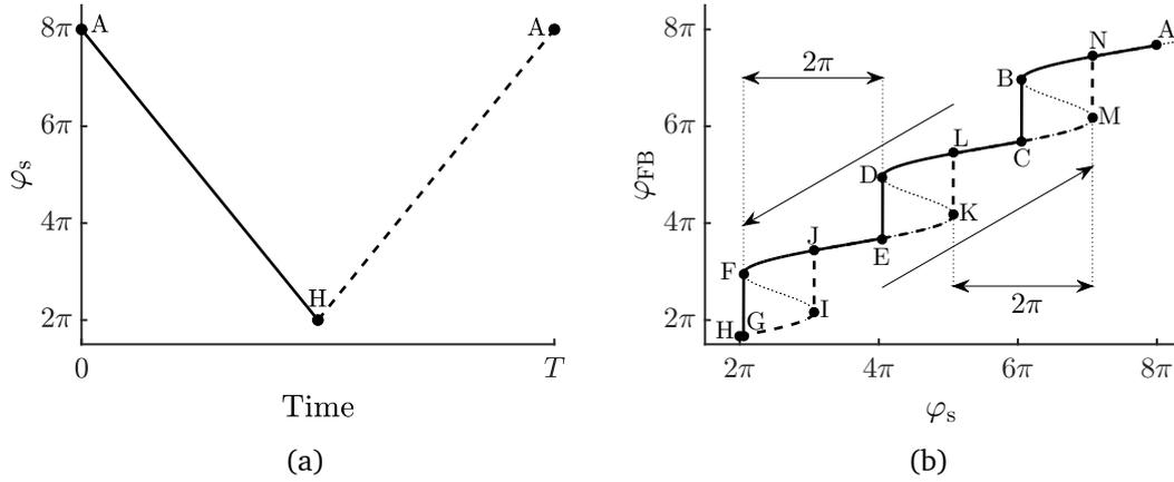
Figure 2.7: Plot (a) show the phase stimulus  $\varphi_s$  is modulated in triangle waveform with a period  $T$  and plot (b) is the resulting of phase response  $\varphi_{FB}$  with the change of  $\varphi_s$  from  $8\pi$  to  $2\pi$ , the feedback parameter  $C = 3$ , and  $\alpha = 5$ . The thin dotted lines shows the unstable solutions to the excess phase equation, the thick solid and dotted lines trace the locus of solution in plot (b) to the phase stimulus in plot (a).
