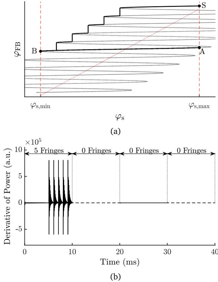
Figure 3.6: Simulation of output power from the rate equations under feedback parameter  $C = 32.16$ . (a) Plot of the phase response  $\varphi_{\text{FB}}$  in function of the phase stimulus  $\varphi_s$ ; the thick solid and broken lines indicate the direction of the phase stimulus during decreasing and increasing respectively. (b) Plot of derivative of output power resulting from the evolution of the phase in (a).
