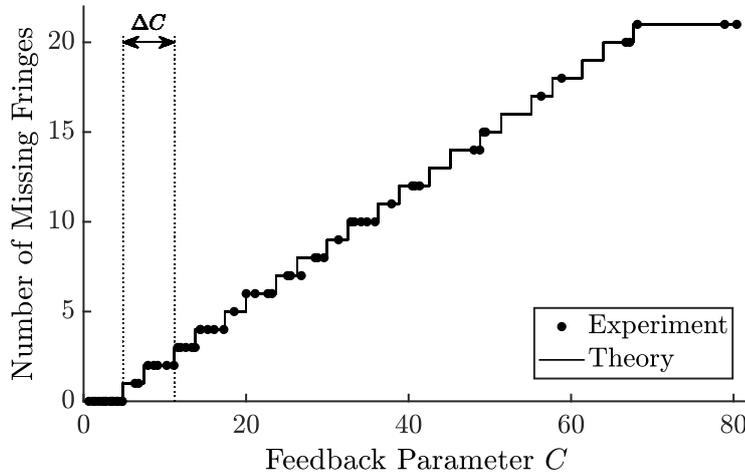
Figure 3.21: The behaviour of the interferometric fringe disappearance and the feedback parameter  $C$ . The thin solid lines show the result of interferometric fringes disappearance in theory and the marker points shows the results of the experiment.
