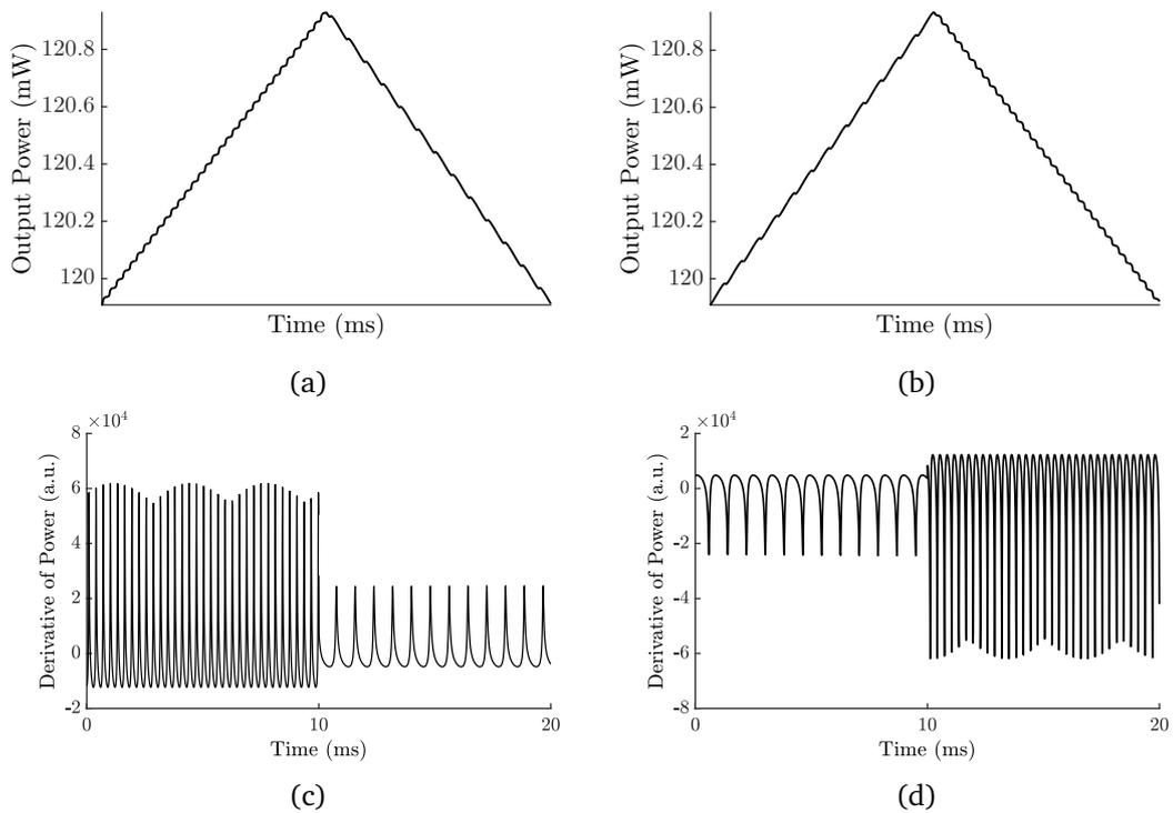
Figure 4.12: Simulation self-mixing power resulting from modulating the phase stimulus in the triangle waveform under the feedback parameter  $C = 0.7$  in different velocity directions. (a) In the clockwise direction with the speed  $v = +2$  mm/s. (b) In the anticlockwise direction with the speed  $v = -2$  mm/s.
