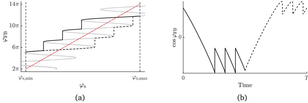
Figure 2.9: Numerical simulation with  $12\pi$  phase stimulus's amplitude modulation. Plot (a) is the phase behaviour under different feedback parameters  $C = 10$ . Plot (b) is the result of derivative of output power which correspond to (a).
