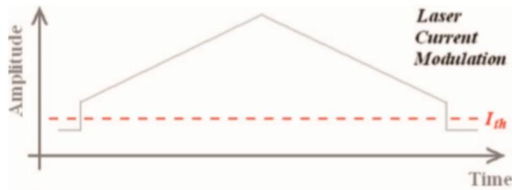
Figure 1.19: The shape of laser current modulation [9].
