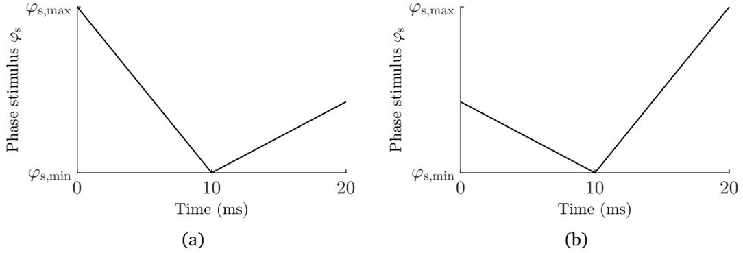
Figure 4.8: Simulation laser phase stimulus for the rotating target. (a) In the clockwise direction with the speed  $v = +0.35$  mm/s. (b) In the anticlockwise direction with the speed  $v = -0.35$  mm/s.
