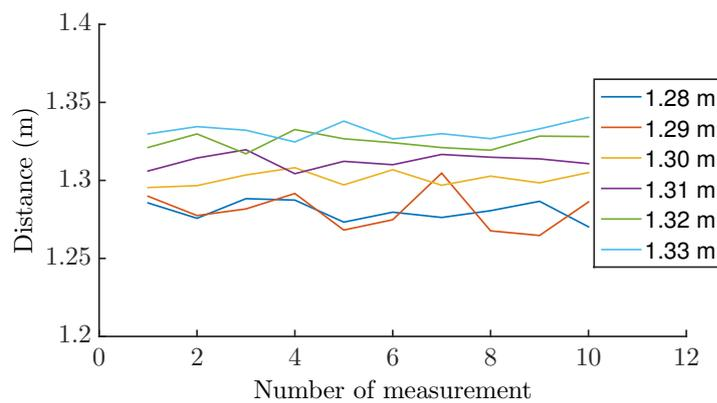
Figure 4.29: Distance measurements resulting from the SMI triangular frequency sweep ranging from 128 cm to 133 cm when the target rotates.
