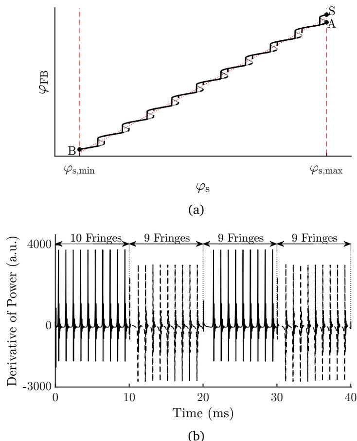
Figure 3.4: Simulation of output power from the rate equations under feedback parameter  $C = 2.20$ . (a) Plot of the phase response  $\varphi_{FB}$  in function of the phase stimulus  $\varphi_s$ ; the thick solid and broken lines indicate the direction of the phase stimulus during decreasing and increasing respectively. (b) Plot of derivative of output power resulting from the evolution of the phase in (a).
