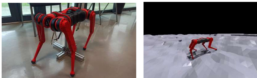
Figure 4.23: Left: The real Sassa robot. Right: The Sassa robot in the IsaacGym simulation learning to traverse a rough slope terrain.
