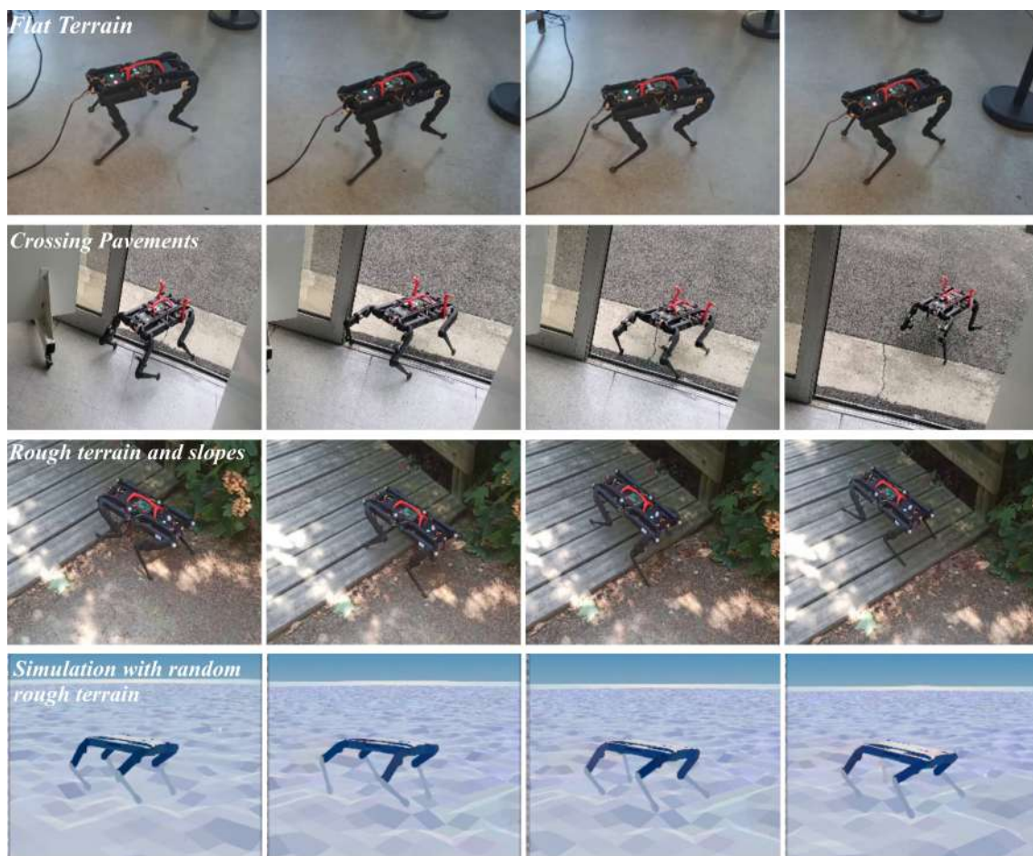
Figure 4.14: Snapshots of the Solo12 quadruped in real settings and in simulation driven by a reactive controller learned through deep reinforcement learning. With learned controllers, the robot can traverse various outdoor environments with slopes and rough ground, full video: https://youtu.be/t-67qBxNyZI .
