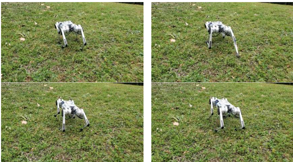
Figure 5.12: We see the robot's right hind leg slipping while Mini-Cheetah is walking on the wet grass. However, the policy is able to recover and keep the robot from falling. Video available here: https://youtu.be/B92HB964xq8?si=C5jS1SsEtIbfdWqM .
