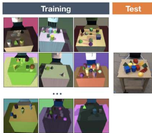
Figure 2.5: Randomizing visual properties of the testing environment as well as the physical location and orientation of the camera and objects. Figure extracted from [Tob + 17].
