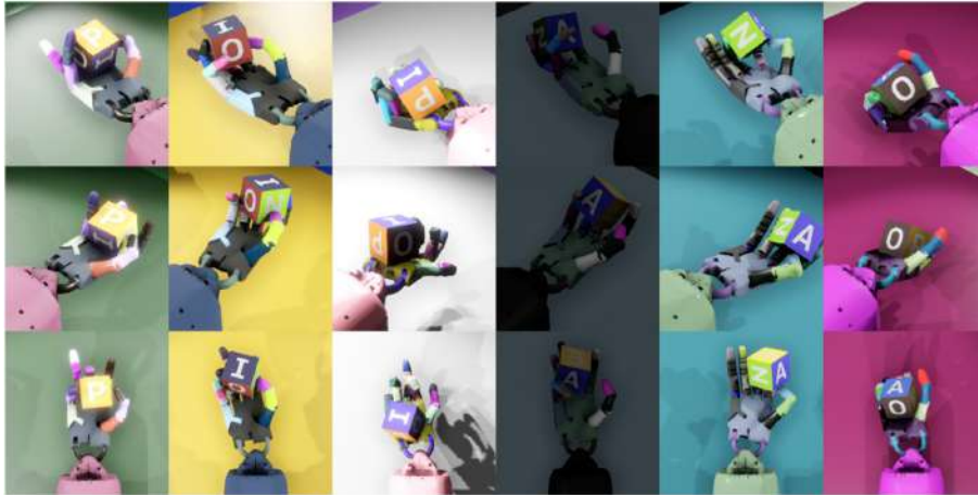
Figure 2.6: Simulating different visual appearances of the same task. Figure extracted from [And + 18].
