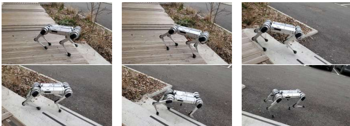
Figure 5.10: Snapshots of the Mini-Cheetah going down a set of stairs in a robust manner without losing balance or falling. Video available here: https://youtu.be/B92HB964xq8?si=C5jS1SsEtIbfdWqM .
