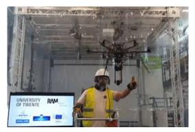
(d) The human signals his intention to start the interaction. At this point, the physical interaction layer of the robot control framework is enabled.
