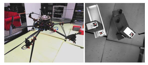
Figure 5.4: On the left, a picture of the fully-actuated hexa-rotor used in the experimental validation, while on the right a picture taken from the onboard camera. In the latter image, the bricks and the placing location are shown. Their successful detection is marked with a red dot displayed over their fiducial markers.
