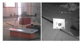
(d) The robot is almost in contact with the placing board and the AruCo tag is still within the camera FoV.
