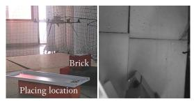
(a) The robot scans the area searching a brick to pick. On the right, no bricks appear within the frame acquired by the onboard camera.
