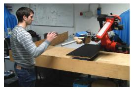
A robot is handing over a tool to a human. Courtesy of [Aleotti, 2012].
