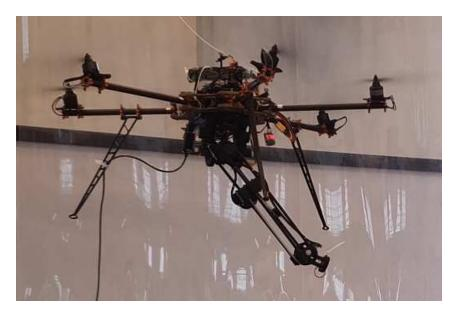
Figure 5.9: A picture of the aerial manipulator adopted in the H2R handover experiment.
