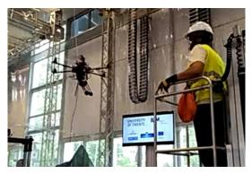
(b) The robot is approaching the operator by moving closer and heading the EE towards the scaffolding.
