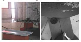
(e) The robot is in contact with the object. The interaction is regulated by means of the physical interaction module.
