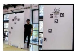
(b) On the left, the wooden panel board utilized as user avatar, and the human operator moving it. On the right, a zoom-in image on the several fiducial markers attached to the board.
