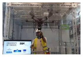
(b) The robot is compliant and moves accordingly to the human pushing force.
