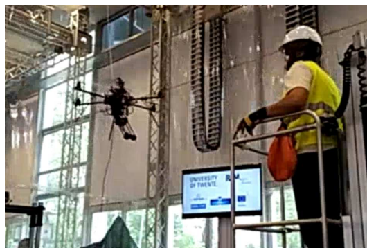
(b) The robot is approaching the operator by moving closer and heading the EE towards the scaffolding.
