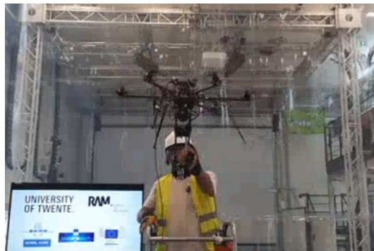
(b) The robot is compliant and moves accordingly to the human pushing force.
