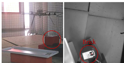
(b) The robot has detected a brick, which is highlighted with a red circle. A successful object detection is marked through a small red dot on top of the identified fiducial marker.
