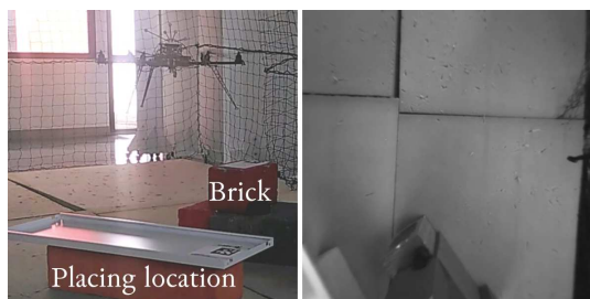
(a) The robot scans the area searching a brick to pick. On the right, no bricks appear within the frame acquired by the onboard camera.
