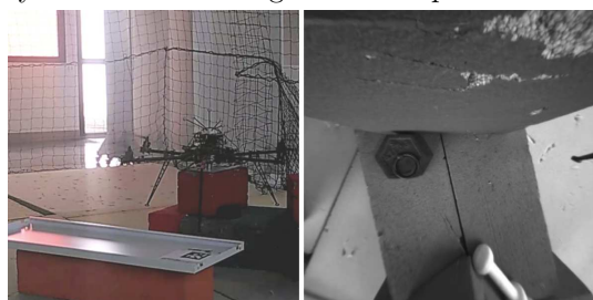
(e) The robot is in contact with the object. The interaction is regulated by means of the physical interaction module.
