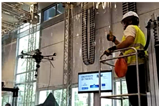
(a) The robot is at its starting location, while a human worker is on a scaffolding signaling the intention to return an object and initiate the handover.
