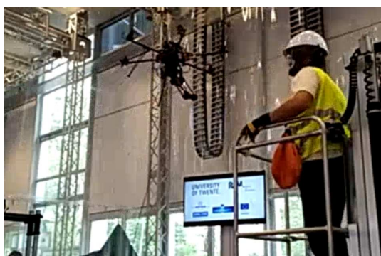
(c) The robot has reached the handover location. It has its EE closer to the user waiting for the human to return the tool.
