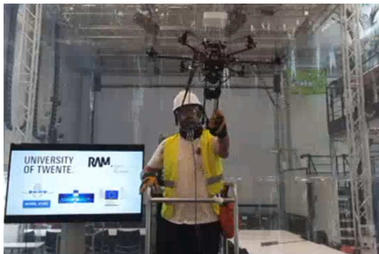
(a) The human worker decides to re-position the robot to a more convenient location matching his preferences by pushing on the robotic arm.
