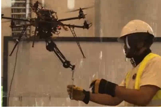
(a) The transferred tool is attached to the robot EE which consists of a simple hook.
