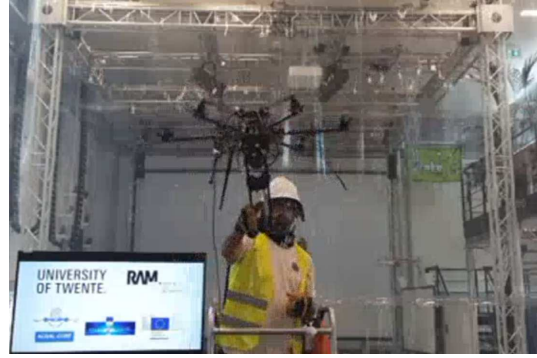
(b) The object transfer has terminated. The human worker decides to move back the robot to the initial handover location.
