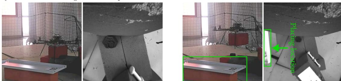
(e) The robot is in contact with the object. The interaction is regulated by means of the physical interaction module.
