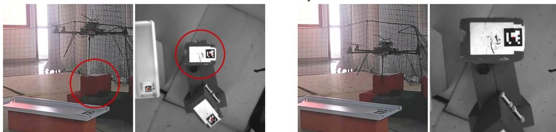
(c) The robot arrives on top of the detected object driven by the velocity commands generated by the visual servoing control loop.
