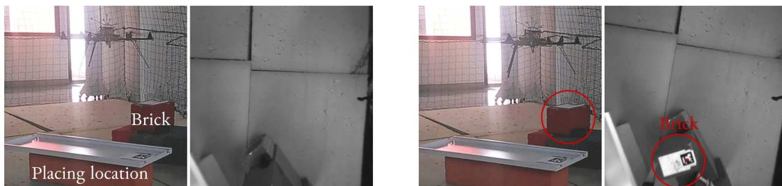
(a) The robot scans the area searching a brick to pick. On the right, no bricks appear within the frame acquired by the onboard camera.
