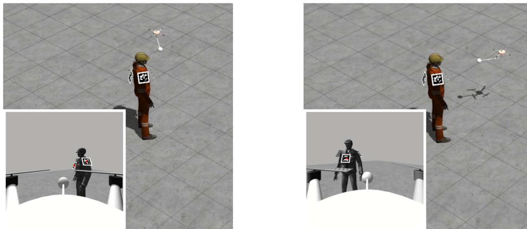
(a) The human stops moving, thus the robot can continue its motion without performing any adaptation.
