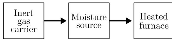
Figure 3.7: Schematic of basic wet thermal oxidation system.
