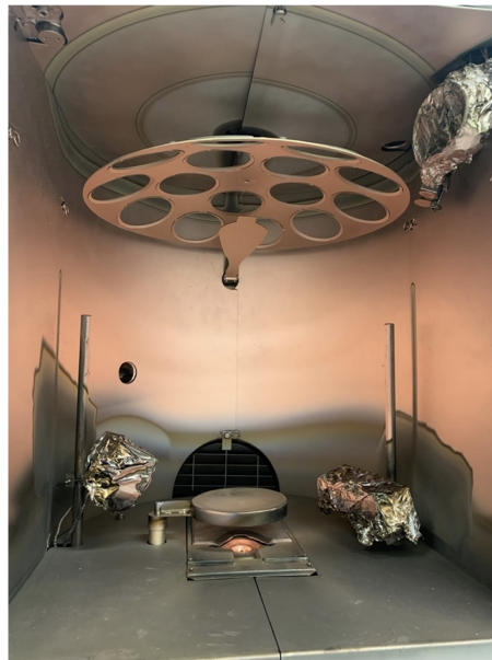
Figure 2.9: Deposition chamber of the EVA 600 PVD machine. The crucible is placed in the lower part whereas the wafers are placed on the top half dome. The whole chamber is put under vacuum during the process.
