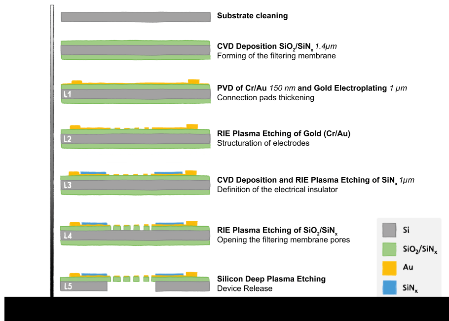
Figure 2: Schematic representation of the steps in the microfabrication process for devices with integrated electrodes on a silicon supporting structure (diagrams are not to scale).
