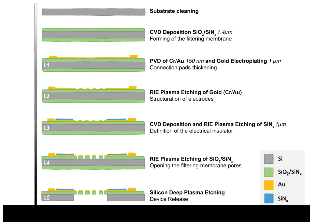
Figure 3.4: Schematic representation of the steps in the microfabrication process for devices with integrated electrodes on a silicon supporting structure (diagrams are not to scale).
