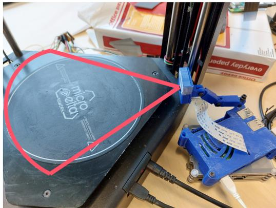
FIGURE A.2: Bed Camera Setup
