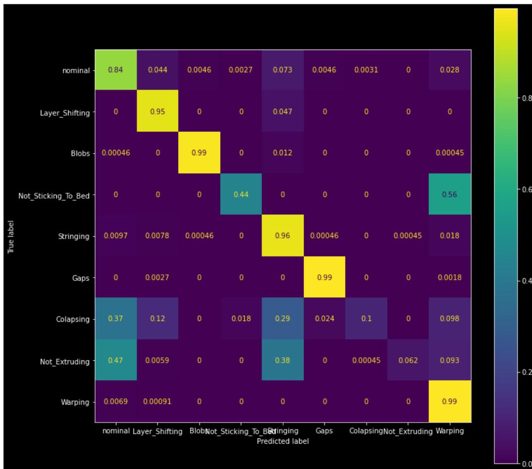
FIGURE 5.13: Confusion Matrix of the Decision Tree Trained by DT4X on the 3D Printer Dataset
