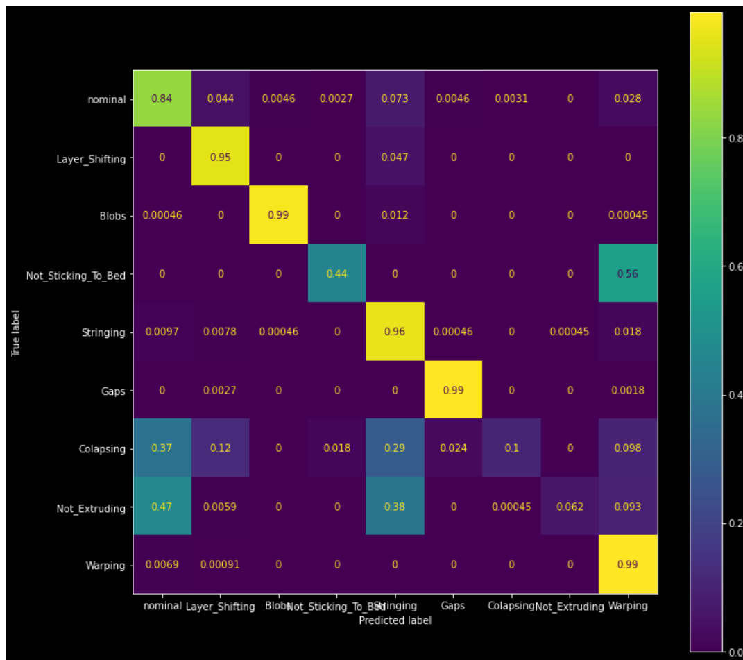
FIGURE 5.13: Confusion Matrix of the Decision Tree Trained by DT4X on the 3D Printer Dataset
