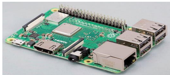
Figure 19. Raspberry Pi 3b+.
