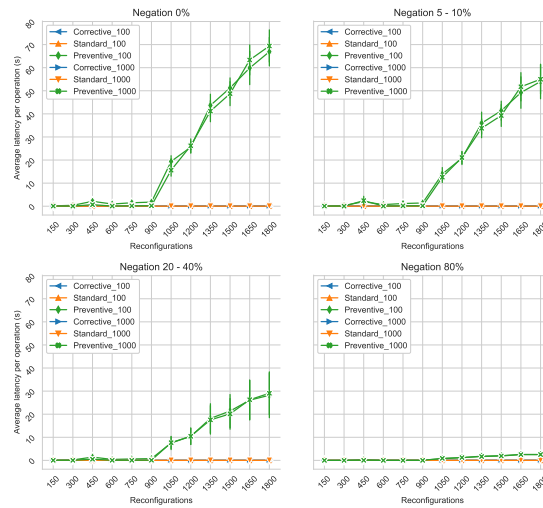
Figure 4.9: The latency variation per VNF-FG reconfiguration operations
