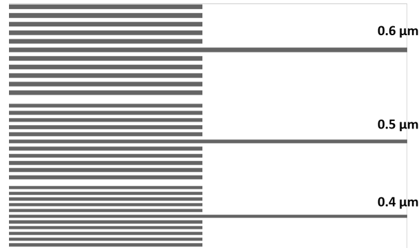
Figure 3.13: Snippet of a test pattern fabricated on n-doped silicon wafers and used to optimize the microfabrication parameters. The width of the lines and gaps varies from 0.1 \mu\text{m} to 5 \mu\text{m} .
