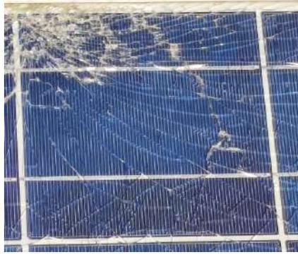
Figure 2.18: Example of Cell crack
