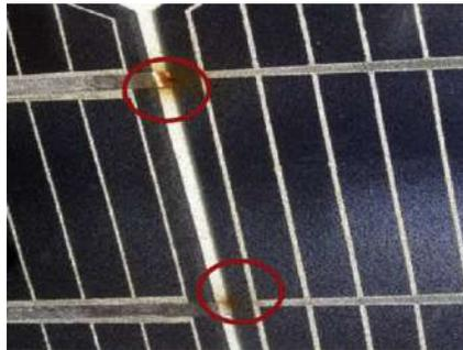
Figure 2.38: Example of Ribbon and Solder Bonds Degradation and Broken Interconnect (R and SB) [Rajput 2019]
