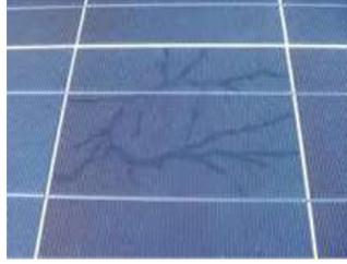
Figure 6.1: Example of snail trail/track fault
