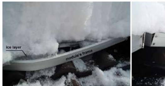
Figure 2.23: Example of Frame breakage [Köntges 2014b]
