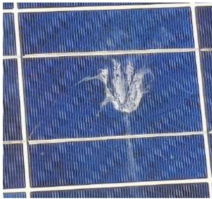
Figure 2.28: Example of Dust and Soiling
