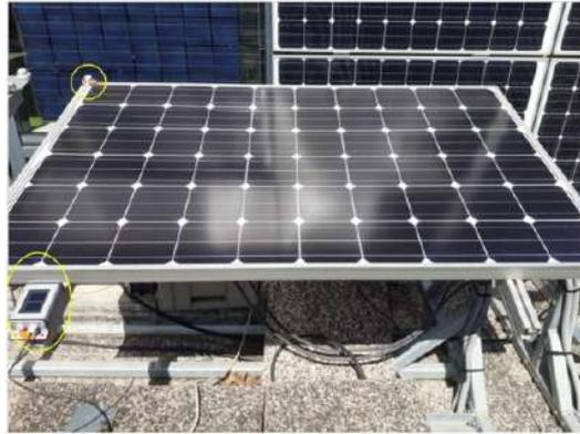
Figure A.7: Positioning of sensors on the panel
