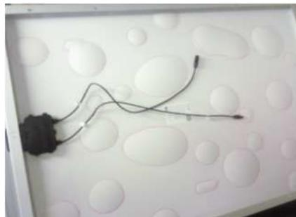
Figure 2.25: Example of Back sheet adhesion loss (BSAL) [de Oliveira 2018]
