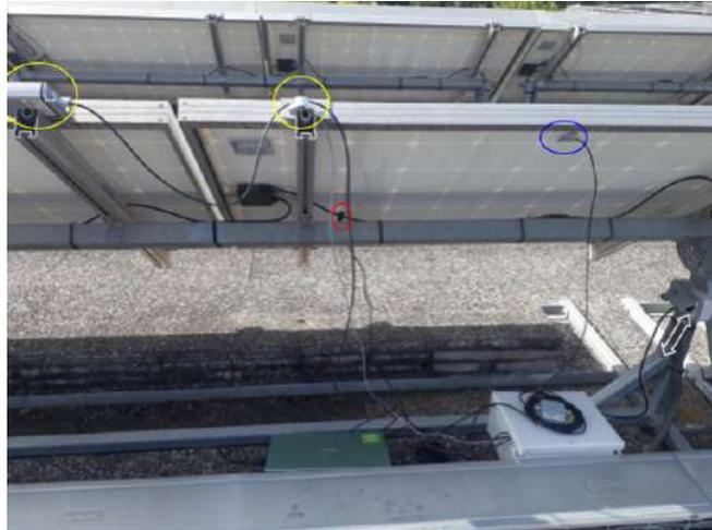
Figure A.1: External connection of the sensors: Irradiance (yellow), Temperature (blue), Current (red) and Electrical power supply (white arrow)
