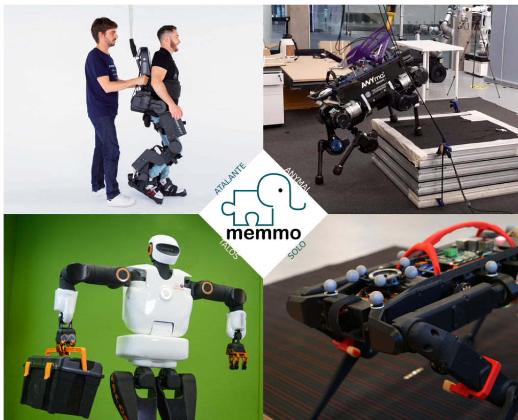
Figure 2.3 – Illustration of the robotic platforms involved in the Memmo project (Atalante, ANYmal, TALOS, and Solo) [67].
