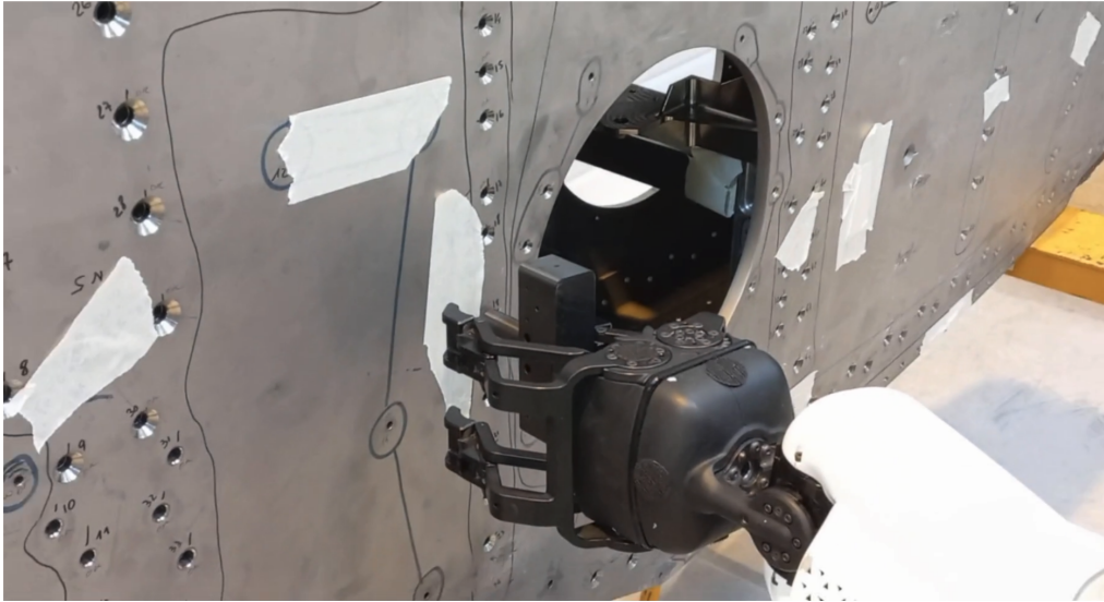
Figure 7.1 – Deburring task, high precision for a fine insertion into a hole using WBMPC on a torque controlled robot.
