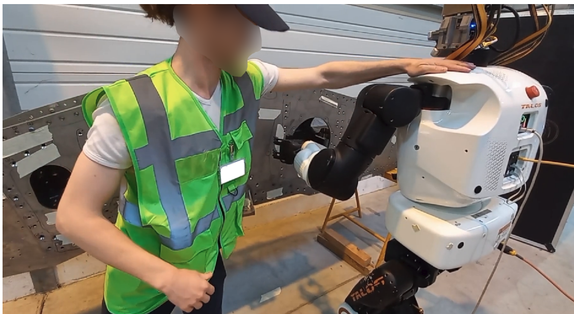
Figure 7.4 – Fine insertion task by a torque-controlled robot in an Airbus factory. The torque control allows a human to interact safely with the robot during movement.
