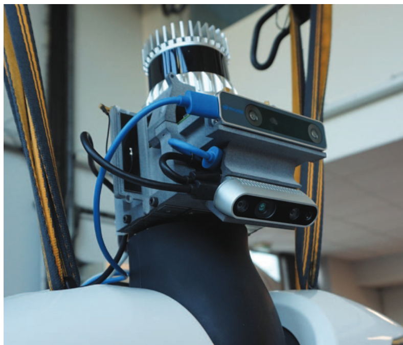
Figure 2.5 – The modified head of Pyrène with a LIDAR (top) and two cameras (middle and bottom) [150].
